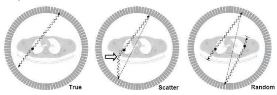
**Figure**: Different types of events in PET measurement. Figure adapted from [1].
